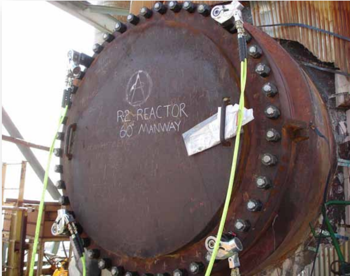
60" R-2 REACTOR MANWAY Parallel Joint Closure Applied Hands-Free via Remote Control
